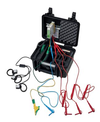
The evaluation software can be accessed quickly and easily via your Internet browser without the need for additional software. The values of the measured variables are stored in the internal memory in different time resolutions from seconds to daily, weekly and monthly values. There is no need for permanent access to the web interface during the measurement.
