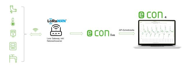
In another option, the LoRa gateways forward the received sensor data to our econ live. In this case, the network server does not run on one of the gateways itself as in the local setup (option 1, see above), but is integrated into the econ live cloud. This makes the processed data available to the econ4 software via an API interface. With this variant, several gateways can be used for the same project, but they do not need to be connected to each other.
