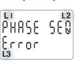
The cabling sequence (L1-L2-L3) is wrong. L1, L2 and L3 icons blink. Invert the voltage wires of 2 phases (phase 1 <> phase 2 or phase 2 <> phase 3). Otherwise, by pressing the «OK» button for at least 5 seconds, the message disappears until the next restart.
