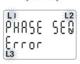
The cabling sequence (L1-L2-L3) is wrong. L1, L2 and L3 icons blink. Invert the voltage wires of 2 phases (phase 1 <> phase 2 or phase 2 <> phase 3). Otherwise, by pressing the «OK» button for at least 5 seconds, the message disappears until the next restart.
